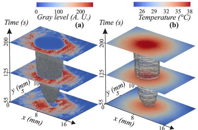
Fig. 3. Two-dimensional characterization of the aperture dilation. (a) Optical aperture: iso-surface for  $I(\vec{r}, t) = 25$  (gray level) recorded with the CCD camera. (b) Thermal aperture: iso-surface for  $\theta(\vec{r}, t) = 36^\circ$  recorded with the thermal camera ( $P_0 = 1$  W,  $w = 5.5$  mm).
